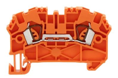
Feed-through terminal, Tension-spring connection, Mounting type: Mounting rail TS 35/7.5, Rated cross-section: 2.5 mm², Width: 5.1 mm, Colour: Orange
