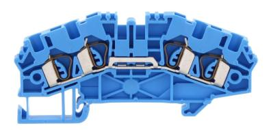
Feed-through terminal, Tension-spring connection, Mounting type: Mounting rail TS 35/7.5, Rated cross-section: 2.5 mm², Width: 5.1 mm, Colour: Blue
