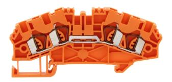
Feed-through terminal, Tension-spring connection, Mounting type: Mounting rail TS 35/7.5, Rated cross-section: 2.5 mm², Width: 5.1 mm, Colour: Orange
