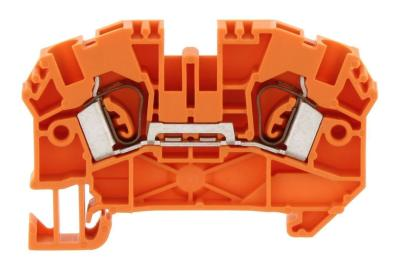
Feed-through terminal, Tension-spring connection, Mounting type: Mounting rail TS 35/7.5, Rated cross-section: 4 mm², Width: 6.1 mm, Colour: Orange
