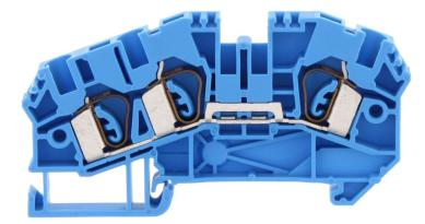
Feed-through terminal, Tension-spring connection, Mounting type: Mounting rail TS 35/7.5, Rated cross-section: 4 mm<sup>2</sup>, Width: 6.1 mm, Colour: Blue
