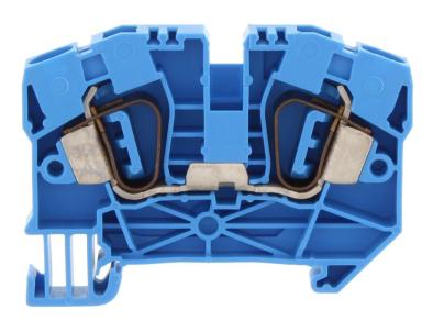
Feed-through terminal, Tension-spring connection, Mounting type: Mounting rail TS 35/7.5, Rated cross-section: 6 mm², Width: 8.1 mm, Colour: Blue
