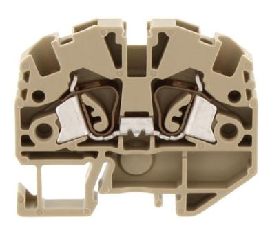
Feed-through terminal, Tension-spring connection, Mounting type: Mounting rail TS 15/5.5, Rated cross-section: 2.5 mm², Width: 5.1 mm, Colour: Beige
