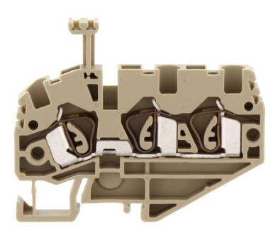
Feed-through terminal, Tension-spring connection, Mounting type: Mounting rail TS 15/5.5, Rated cross-section: 2.5 mm², Width: 5.1 mm, Colour: Beige
