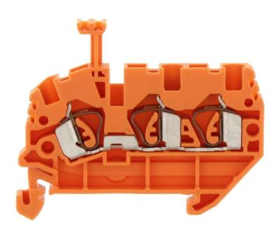
Feed-through terminal, Tension-spring connection, Mounting type: Mounting rail TS 35/7.5, Rated cross-section: 2.5 mm², Width: 5.1 mm, Colour: Orange
