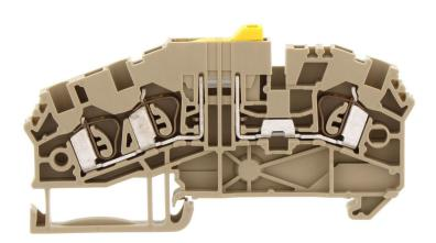
Disconnect-blade terminal, Tension-spring connection, Mounting type: Mounting rail TS 35/7.5, Rated cross-section: 2.5 mm², Width: 5.1 mm, Colour: Beige
